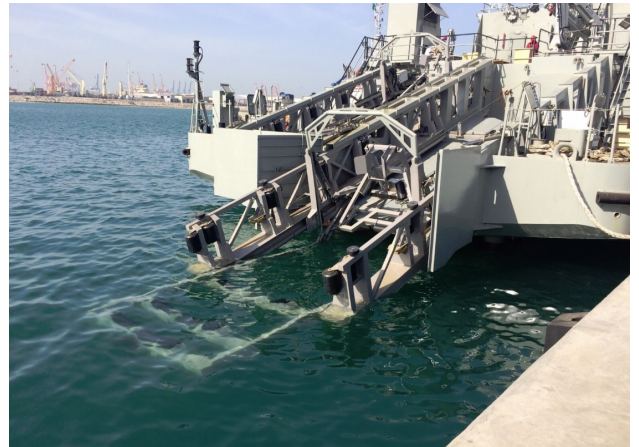
The starboard LARS in its deployment position
